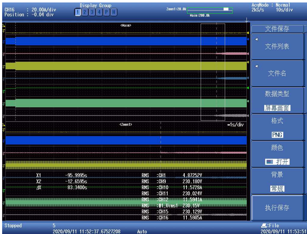
Test 2: All phases reconnection time
