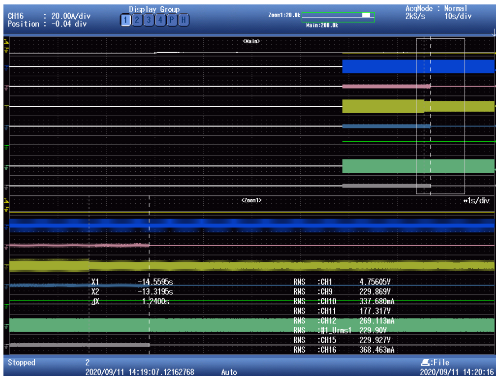
Test 3: Phases L2 disconnection time
