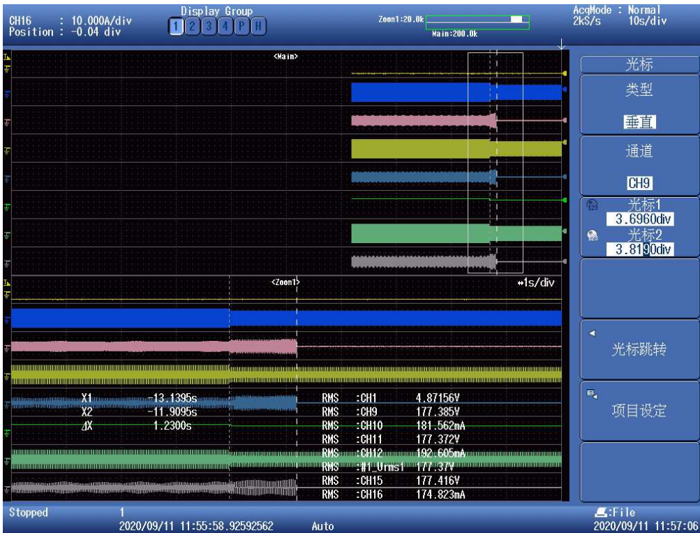
Test 3: All phases disconnection time
