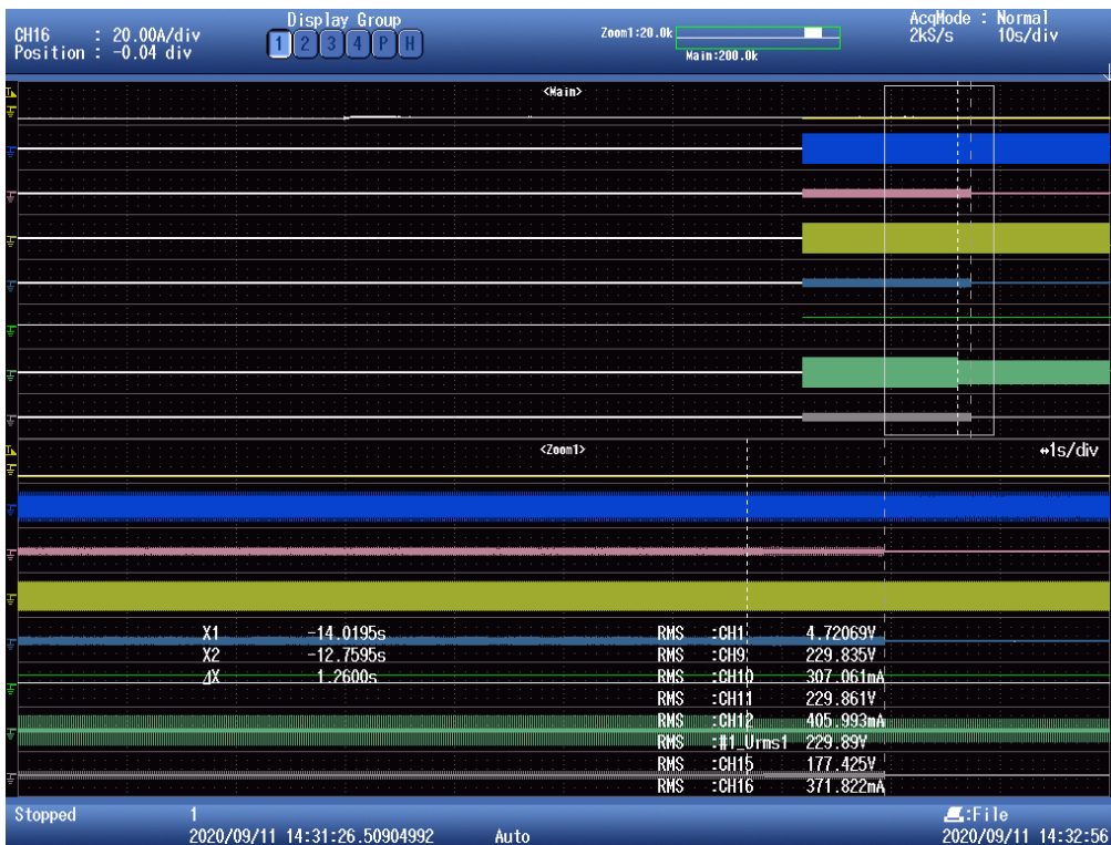
Test 2: Phases L3 disconnection time
