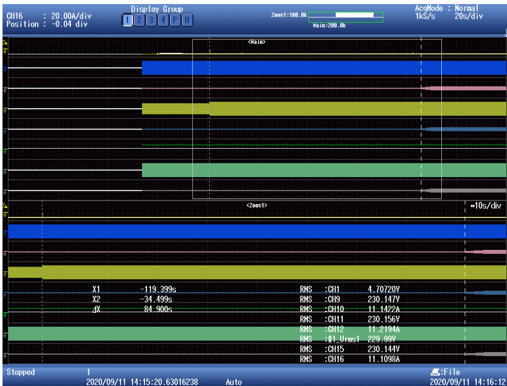
Test 2: Phase L2 reconnection time
