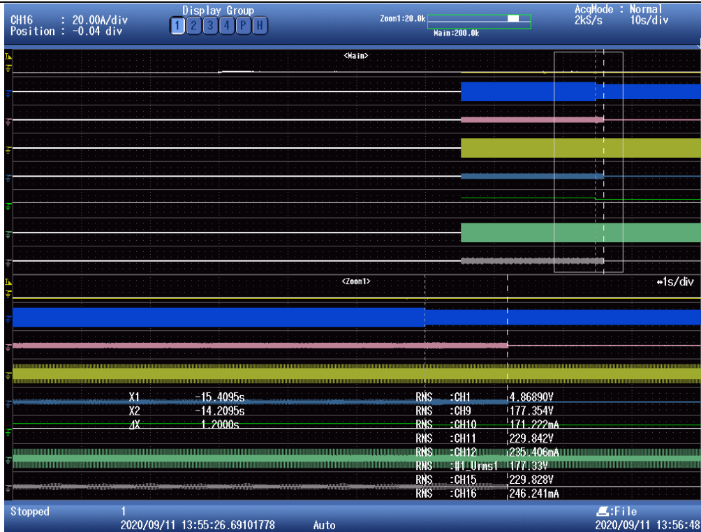
Test 3: Phases L1 disconnection time
