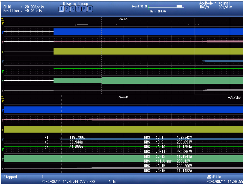
Test 2: Phase L3 reconnection time
