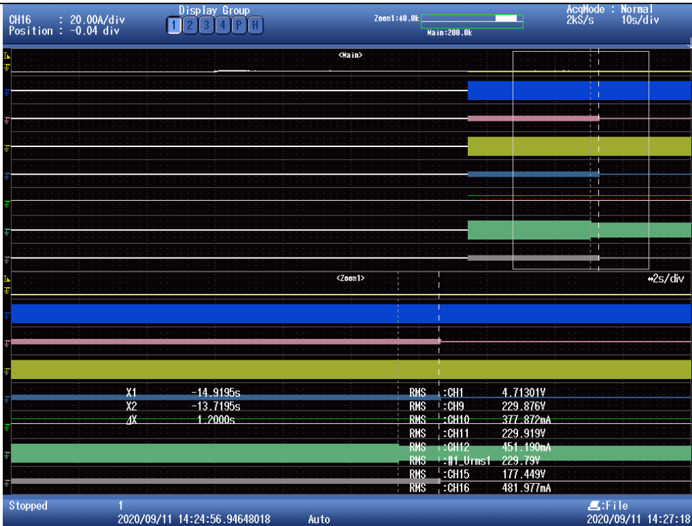
Test 1: Phases L3 disconnection time
