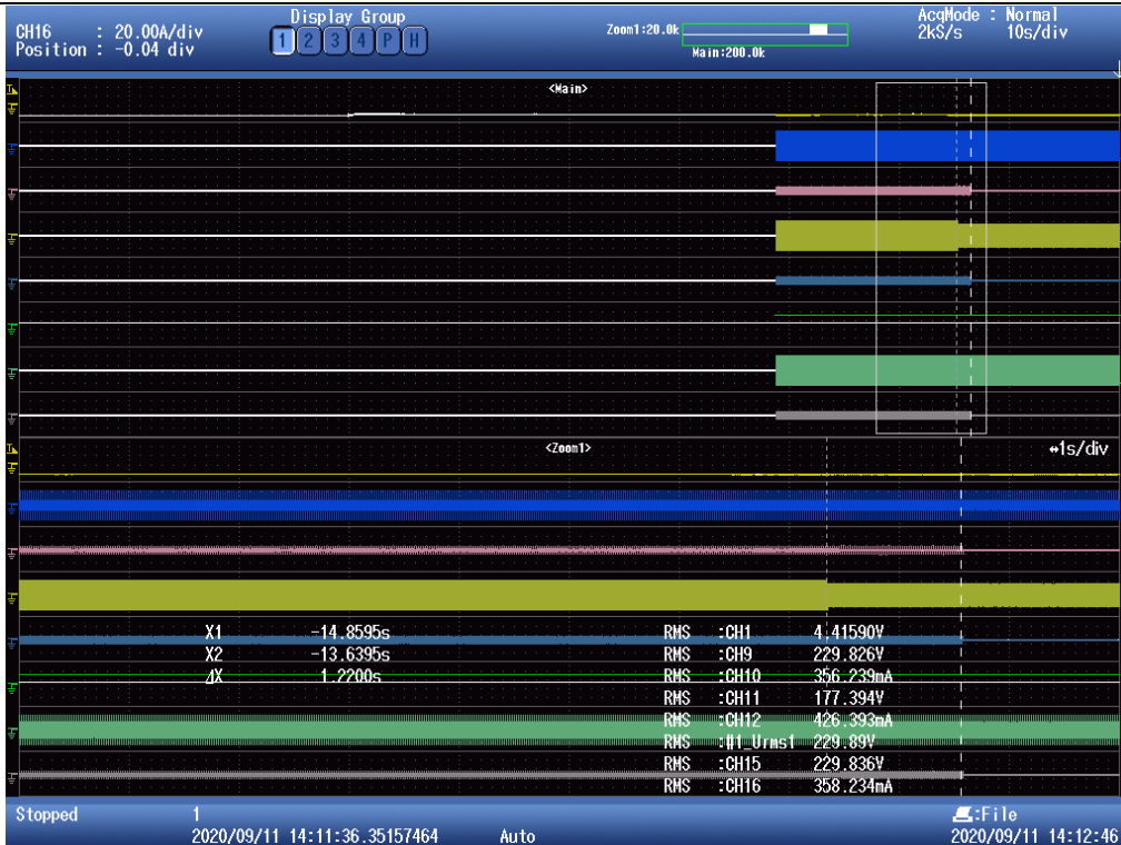
Test 2: Phases L2 disconnection time
