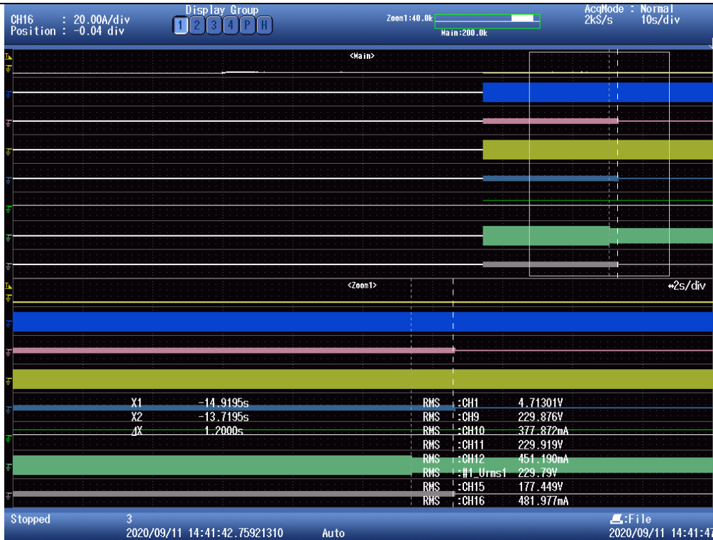
Test 3: Phases L3 disconnection time
