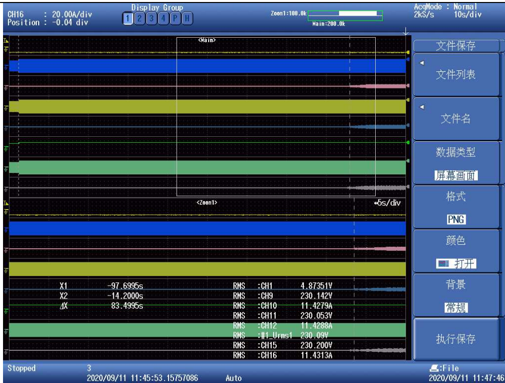
Test 1: All phases reconnection time
